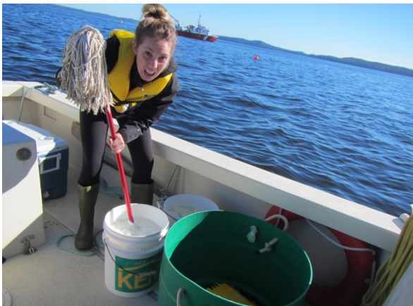
Taryn Minch mixing powdered milk and seawater for a tracer release trial at Navy Island Atlantic salmon farm in the Bay of Fundy, New Brunswick (photo credit: Adena Peters).
